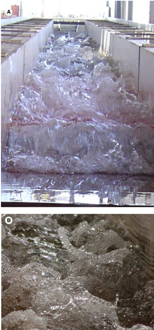
Fig. 1. Advancing flood wave down an initially dry stepped cascade (present study). (A) Q(t=0+) = 0.065 \text{ m}^3/\text{s} , step 16, h = 0.0715 \text{ m} , l = 1.2 \text{ m} , looking upstream at the advancing surge (Courtesy of Chye-guan SIM, and Chee-chong TAN). (B) Air–water flow structure just behind the flood wave leading edge ( Q(t=0+) = 0.065 \text{ m}^3/\text{s} , step 16, h = 0.0715 \text{ m} , l = 1.2 \text{ m} , looking upstream).
