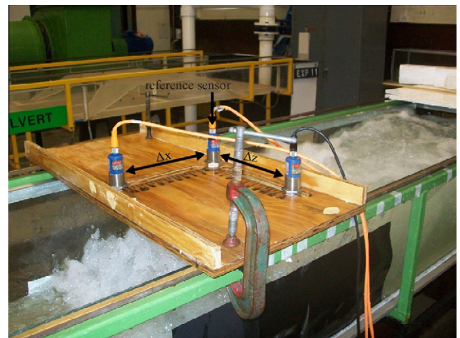
Fig. 2. Experimental setup with three acoustic displacement metres and definition of the longitudinal and transverse separation distances \Delta x and \Delta z – flow from left to right: d_1 = 39.5 mm, x_1 = 1.50 m, Fr_1 = 5.1 , Re = 1.3 \times 10^5 .
