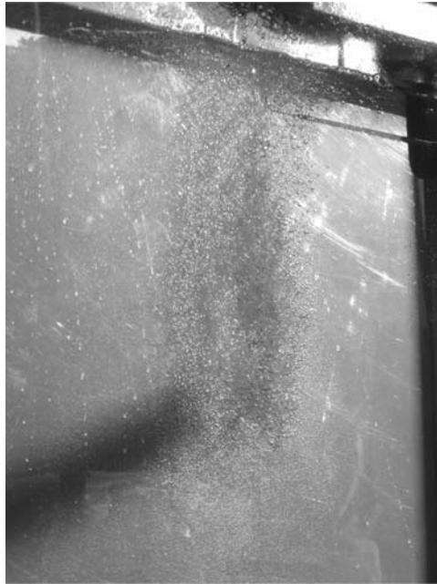
Figure 9. Air bubble entrainment at circular plunging jet in seawater d_n = 0.0125 mm, x_1 = 0.050 m, V_1 = 2.46 m/s.
