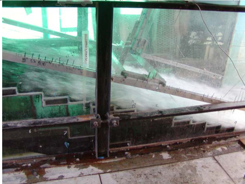
Fig. 1 - Photograph of the experimental facility ( d_c/h = 1.7 , h = 0.05 m, \theta = 15.9^\circ )
