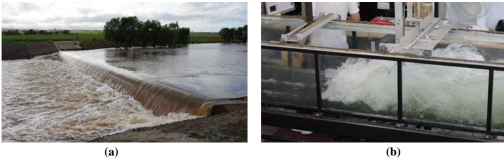
**Figure 1** (a) Hydraulic jump at Joe Sippel weir, Murgon QLD, Australia (5<sup>th</sup> March 2013) –  $Q = 27.0 \text{ m}^3/\text{s}$ ,  $B = 36.34 \text{ m}$ ,  $Re = 7.3 \times 10^5$ ; (b) Experimental hydraulic jump – Flow conditions:  $Q = 0.0812 \text{ m}^3/\text{s}$ ,  $B = 0.5 \text{ m}$ ,  $d_1 = 0.057 \text{ m}$ ,  $x_1 = 1.25 \text{ m}$ ,  $Fr_1 = 3.8$ ,  $Re = 1.6 \times 10^5$ .
