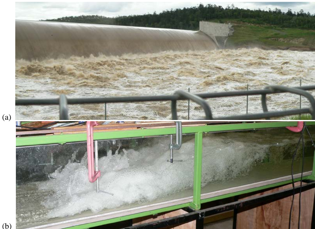
Figure 5 Comparison of air-water flow features between prototype and laboratory model operations of hydraulic jumps; (a) Hydraulic jump stilling basin downstream of Paradise Dam spillway (Australia) in operation on 30 December 2010 (Courtesy of B. Chanson): Q \approx 6,300 \text{ m}^3/\text{s} , F = 8 , R = 2 \times 10^7 ; (b) Laboratory experiment: Q = 0.030 \text{ m}^3/\text{s} , F = 8 , R = 6 \times 10^4
