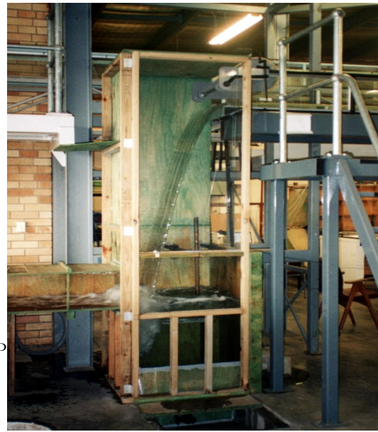
Fig. 2 – Dropshaft in operation with Q=12 L/s
