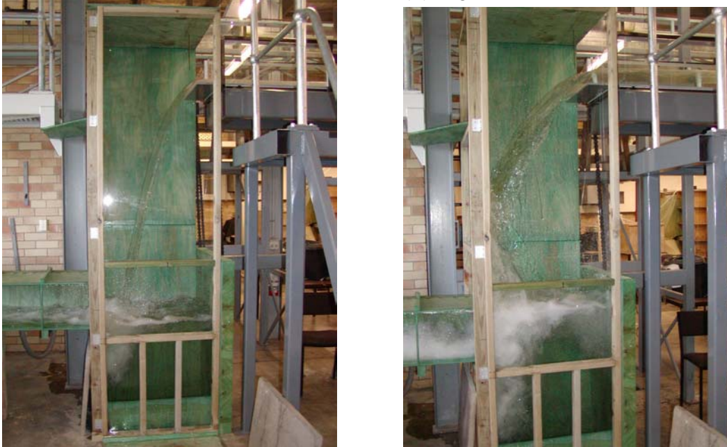
Fig. 2-1 : Rectangular dropshaft in operation (shaft dimensions: 0.76 m × 0.75 m) (A) Regime R1 (B) Regime R3
