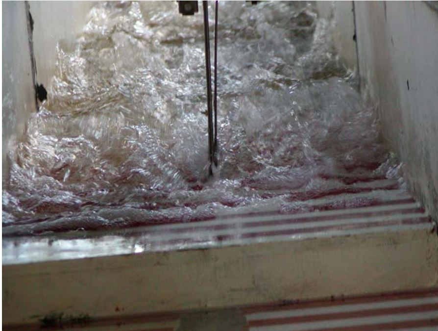
Fig. 1 - Advancing flood wave down a stepped cascade ( h = 0.0715 m, l = 1.2 m) (A) Q(t=0+) = 0.055 m 3 /s, step 16, looking upstream with single-tip conductivity probe array in foreground
