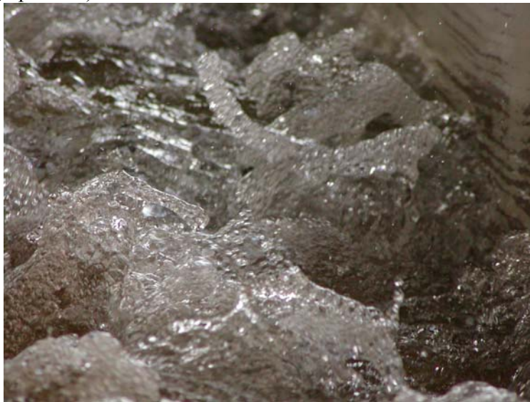
(B) Air-water flow structure just behind the flood wave leading edge ( Q(t=0+) = 0.065 m 3 /s, step 16, looking upstream)
