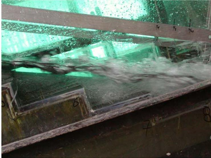
(b) Spray and droplet generation captured with high-shutter speed - Flow from left to right - Configuration 2 with 3 vanes in line ( $d_c/h = 1.1$ )
