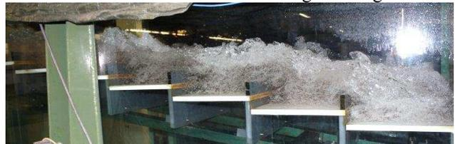
(B) Free-surface instationarities in air-water flows on the pooled stepped spillway:  $\theta = 8.9^\circ$ ,  $h = 0.05$  m,  $q = 0.152$  m<sup>2</sup>/s,  $d_p/h = 2.66$ ,  $Re = 6.0 \times 10^5$
