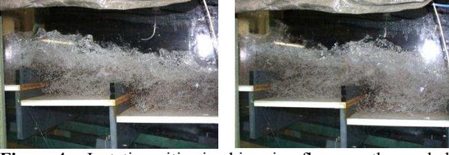
**Figure 4:** Instationarities in skimming flows on the pooled stepped spillway:  $\theta = 8.9^\circ$ ,  $h = 0.05$  m,  $q = 0.122$  m<sup>2</sup>/s,  $d_c/h = 2.3$ ,  $Re = 4.9 \times 10^5$
