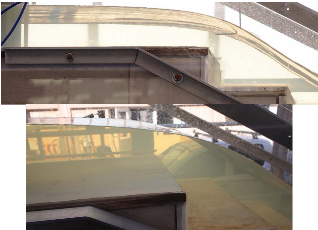
Fig. 1 - Photographs of the free-surface at the downstream end of weir crest (i.e. brink) for H_1/L_{\text{crest}} = 0.18 (Top) and 0.24 (Bottom) with flow direction from left to right - Note the Prandtl-Pitot tube on the right
