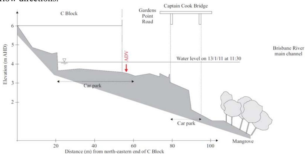
Fig. 4 - Dimensioned transect of the flooded Gardens Point Road and surroundings looking downstream
