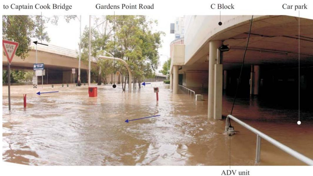
Fig. 2 - Gardens Point Road during the flood on 13 January 2011 at 11:40 looking upstream. Blue arrows show the main flow directions
