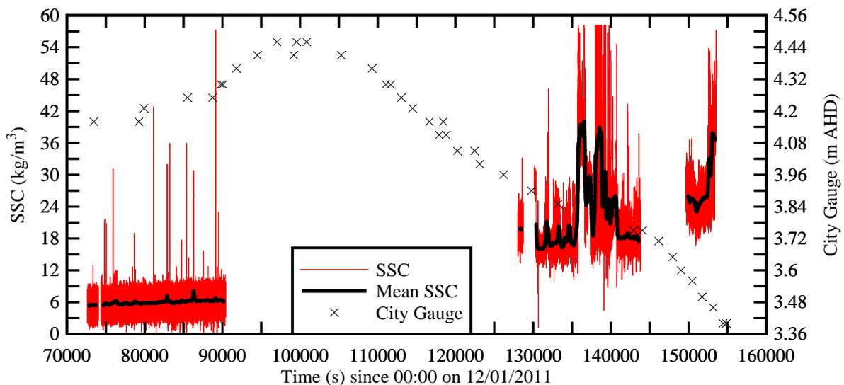
Fig. 8 - Time variations of suspended sediment concentration SSC along Gardens Point Road on 12-13 January 2011
