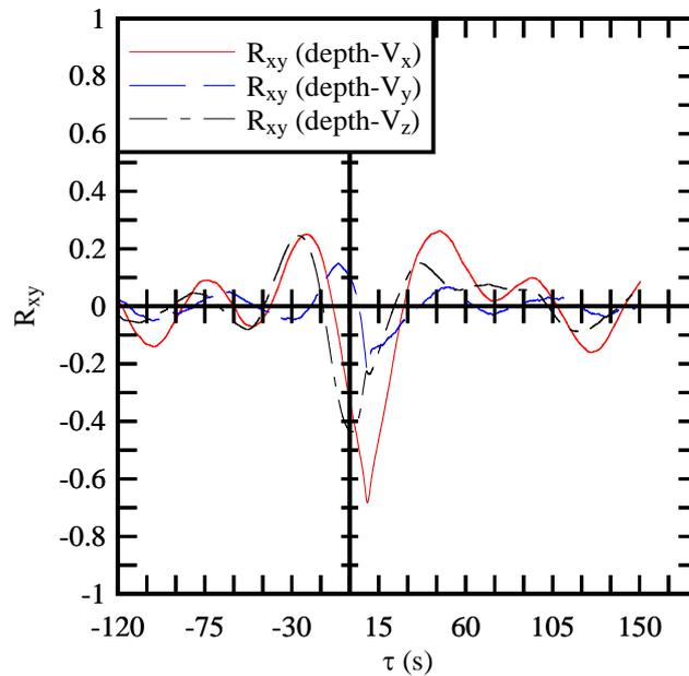
Fig. 7 - Cross-correlation functions between instantaneous water level and velocity component for  $74,000 < t < 89,000 \text{ s}$
