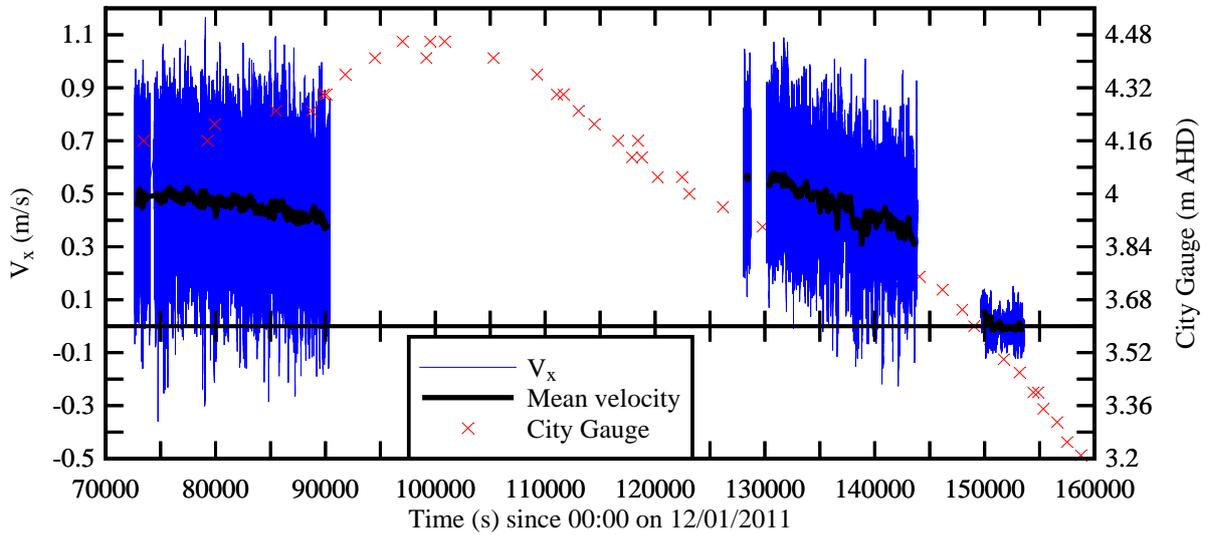
Fig. 6 - Time variations of the longitudinal velocity  $V_x$  along Gardens Point Road during the January 2011 flood - Comparison with the Brisbane River City Gauge data
