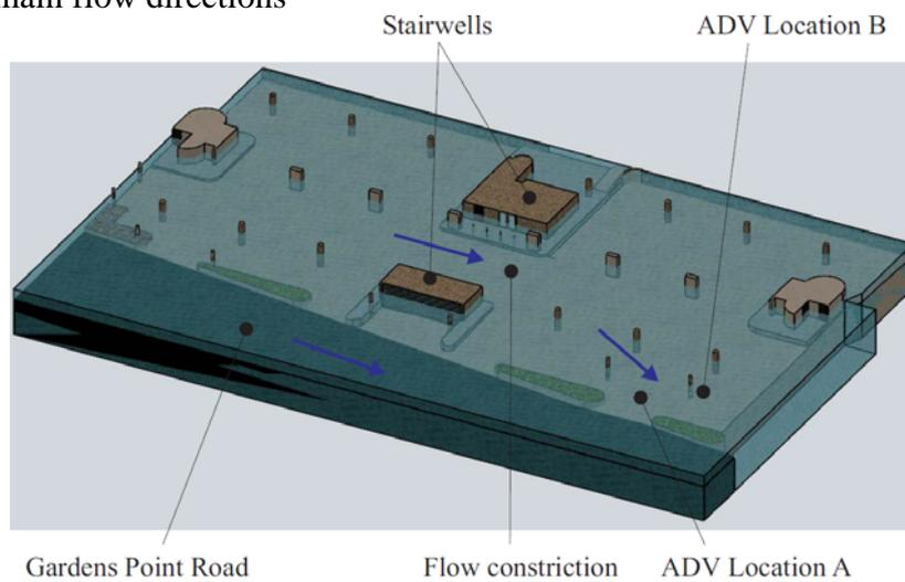
Fig. 3 - CAD sketch of the inundated Gardens Point Road and C Block car park. Blue arrows show the main flow directions.
