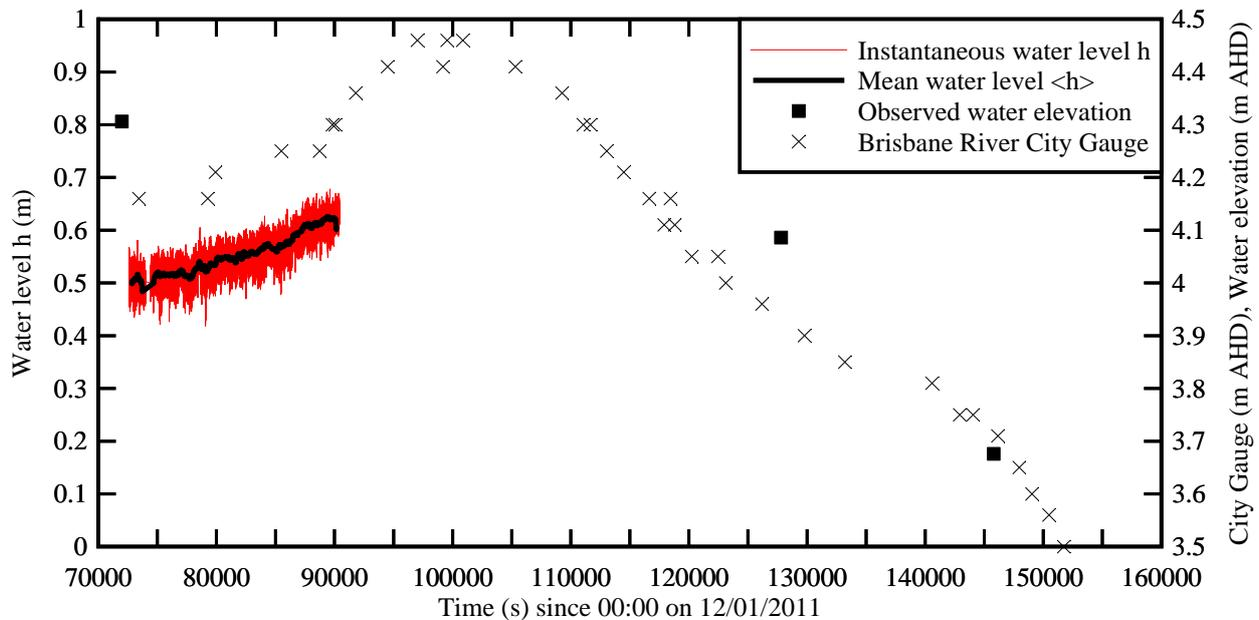
Fig. 5 - Instantaneous and mean water levels. Comparison with City Gauge data and observed water elevation
