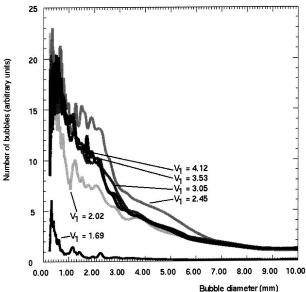
Fig. 10 Bubble-size spectra, jet height  $x_1 = 100$  mm
