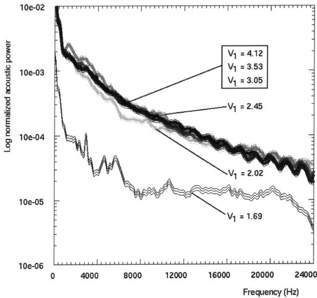
Fig. 9 Acoustic spectra, jet height  $x_1 = 100$  mm
