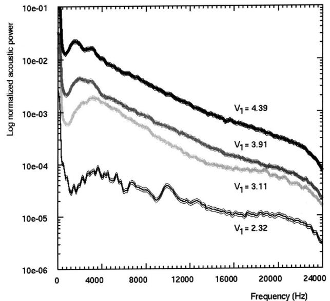
**Fig. 4 Acoustic spectra, jet height  $x_1 = 5$  mm after [16]**
