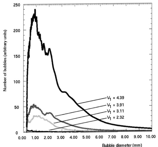
**Fig. 5 Bubble-size spectra, jet height  $x_1 = 5$  mm after [16]**
