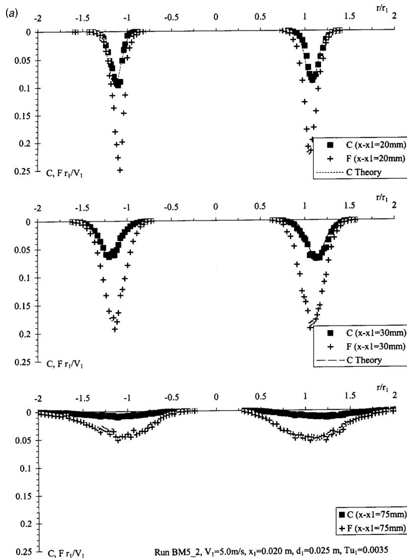
**Fig. 2 Dimensionless distributions of void-fraction and bubble count. Dashed line is solution of Eq. (1).  $Tu_1$  is turbulence intensity based on longitudinal velocity fluctuations at jet impact. (a) Jet height,  $x_1=20$  mm, jet velocity  $V_1=5.0$  m/s,  $Tu_1=0.35\%$ . (b) Jet height  $x_1=100$  mm, jet velocity  $V_1=3.5$  m/s,  $Tu_1=0.39\%$ .**
