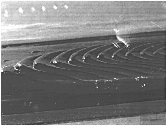
Fig. 10. Man-made instabilities induced after stoppage, during cleanup in the large facility when the reservoir fluid was pushed over the stopped fluid—Test 05, Flow Type II, \theta_b=15^\circ , C_m=15\% , T_o=60 s, and M=3.7 kg. Flow direction from right to left.
