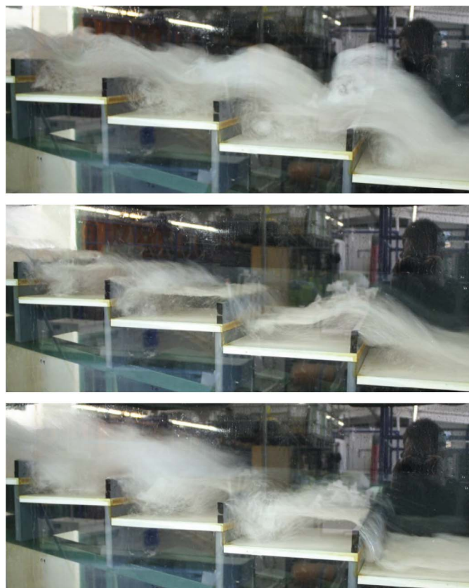
Fig. 3. Jump waves in the transition flow regime on the pooled stepped spillway ( \theta = 8.9^\circ ): d_c/h = 1.20 ; q_w = 0.046 \text{ m}^2/\text{s} ; R = 1.8 \times 10^5
