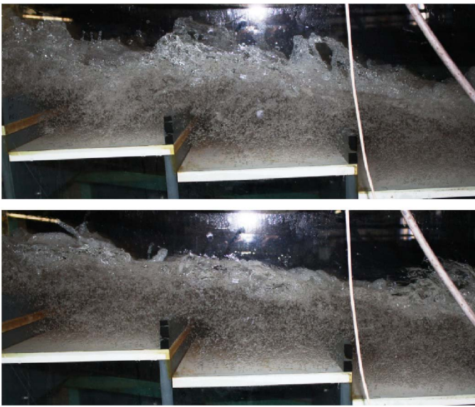
Fig. 4. Instabilities in the skimming flow regime on the pooled stepped spillway ( \theta = 8.9^\circ ); d_c/h = 2.66 ; q_w = 0.152 \text{ m}^2/\text{s} ; R = 6.0 \times 10^5
