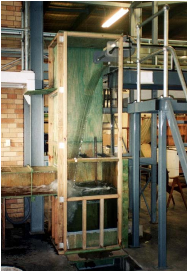
Fig.2 - Dropshat in operation with Q=12 L/s
