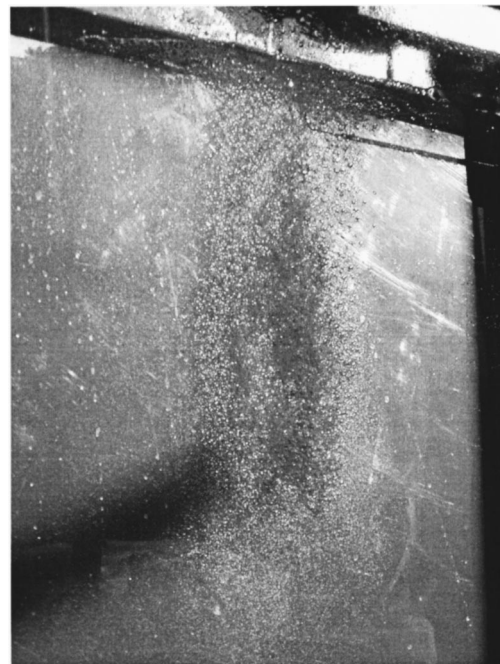
FIG. 2. Photographs of air entrainment at circular plunging jet in seawater: D_n = 0.0125 mm, h = 0.050 m, V_j = 2.46 m/s, Fr_j = 7.2 —Underwater view, flow from top to bottom (after Chanson et al. , Ref. 5).
