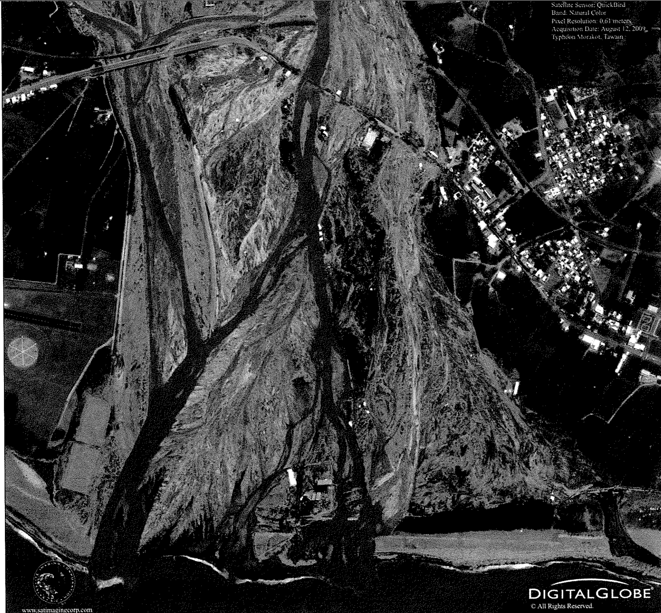
Figure 2. Photograph of the Taimali River mouth on 12 August 2009 (courtesy of Satellite Imaging Corporation). Note the devastated Taimali township on the right and the damaged railway bridge (top), and road <42> bridge (just beneath), as well as the airfield on the bottom left. From left to right, the distance is about 2.3 km.
