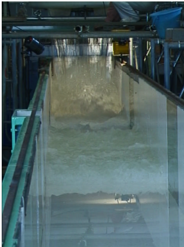
Fig. 4 - Wave propagation in the channel - Run No. 3, d_1 = 0.03 m (A) Wave propagation ( t \sim 3.5 s, x_s \sim 8 m)
