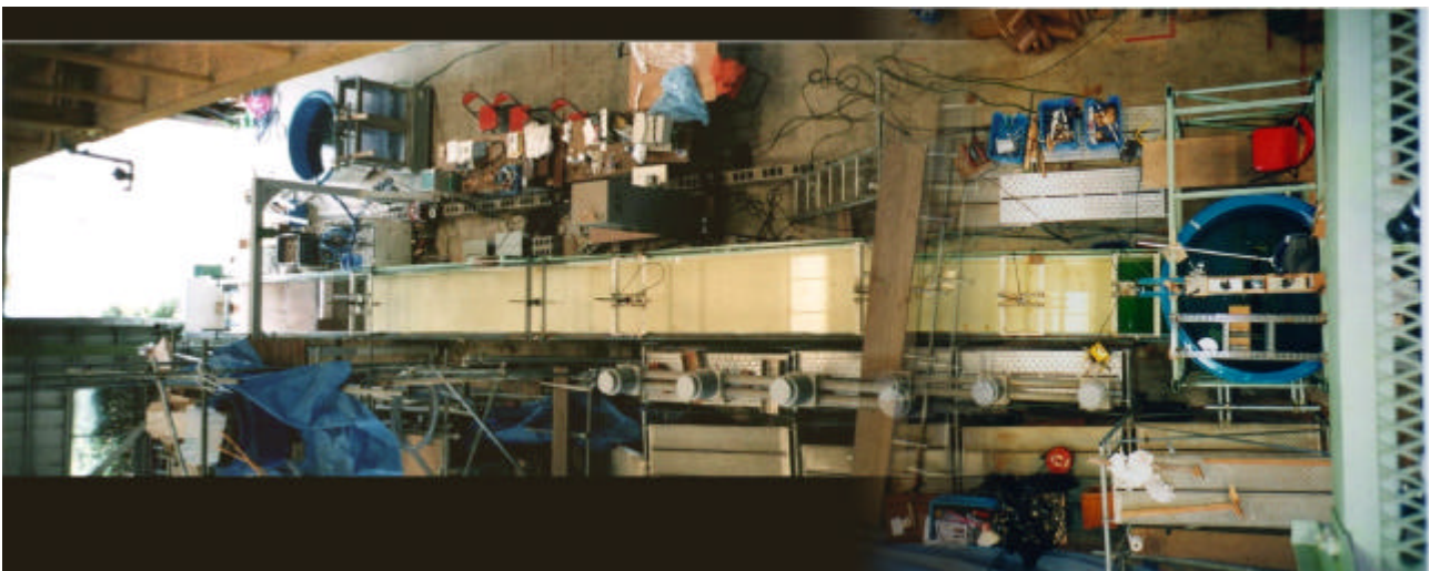
(B) Top view of the flume, with the circular water reservoir on the right of the photograph
