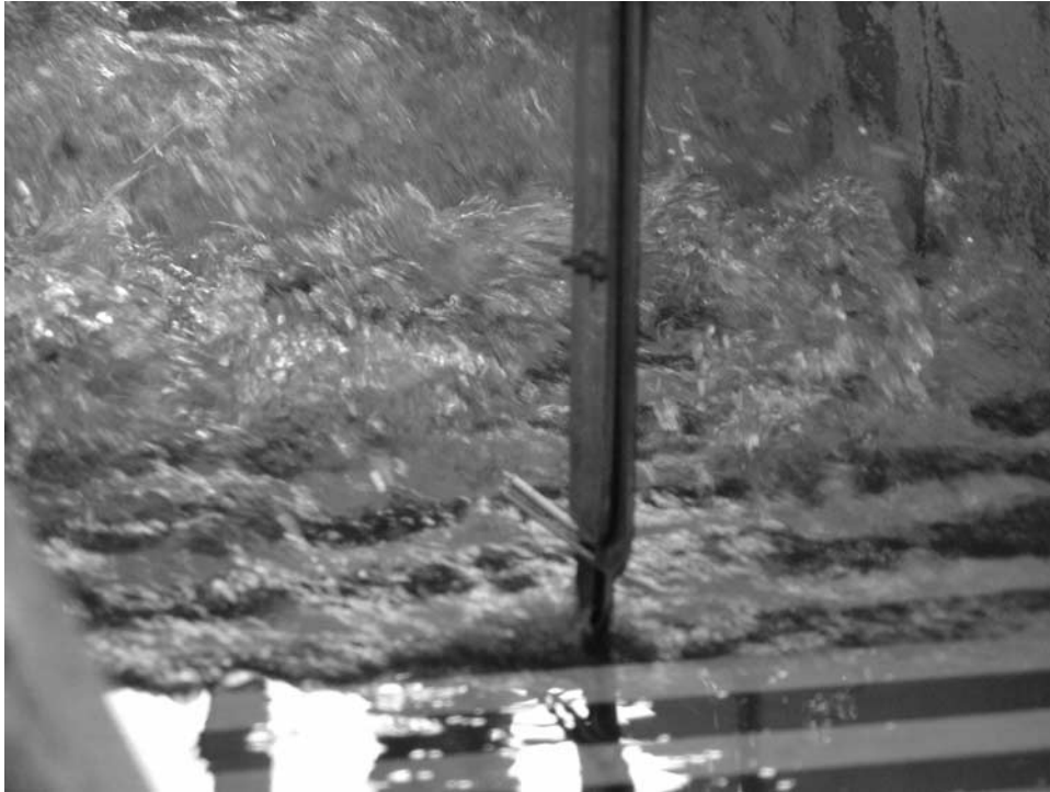
Figure 2. Advancing surge front and conductivity probes. Experiment series 2 ( Q(t = 0+) = 0.075 \text{ m}^3/\text{s} , d_o = 0.297 \text{ m} , step 10, h = 0.0715 \text{ m} ). Advancing surge front just touching the conductivity probe sensors. Looking upstream. See color version of this figure in the HTML.
