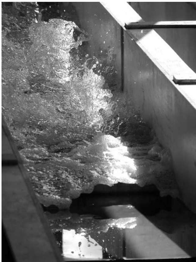
Figure 1b. Experimental facility at the University of Queensland: Experiment series 2 ( Q(t = 0+) = 0.065 \text{ m}^3/\text{s} , step 10, h = 0.0715 \text{ m} ). Surge front taking off, flow direction from top left to bottom right. Note the “white waters” at the leading edge. See color version of this figure in the HTML.
