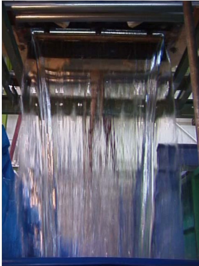
Fig. 7-11 - Photograph of the free-falling jet beneath a large two-dimensional orifice flow ( l = 0.070 m, B = 0.750 m) at the bottom of a large circular tank (CHANSON et al. 2002) - Frontal view of the full jet width (0.750 m)
