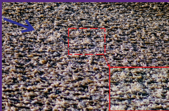
Figure 3: Details of high-velocity self-aerated free-surface flow - High-shutter speed photograph (1/8,000 s) for Re = 3 \times 10^6 . Flow direction from top left to bottom right.
