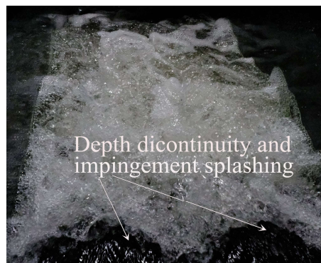
Figure 4. Details of the impingement edge at the jump toe. Looking downstream – Flow conditions: Q = 0.0883 \text{ m}^3/\text{s} , d_1 = 0.07 \text{ m} , x_1 = 1.1 \text{ m} , Fr_1 = 3.045 , Re = 1.97 \times 10^5 [Photo details: camera Fujifilm X-T30 II, shutter speed 1/500 s, 18mm focal length, f/20]
