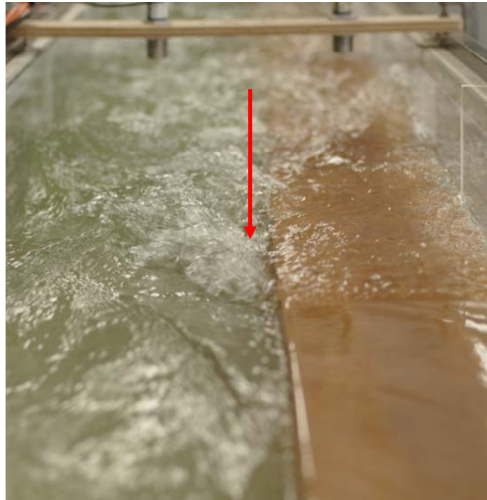
Figure 7. Dyke overtopping by an advancing bore and wake motion (Arrow) behind the bore front at the edge of the dyke - Bore motion from background to foreground
