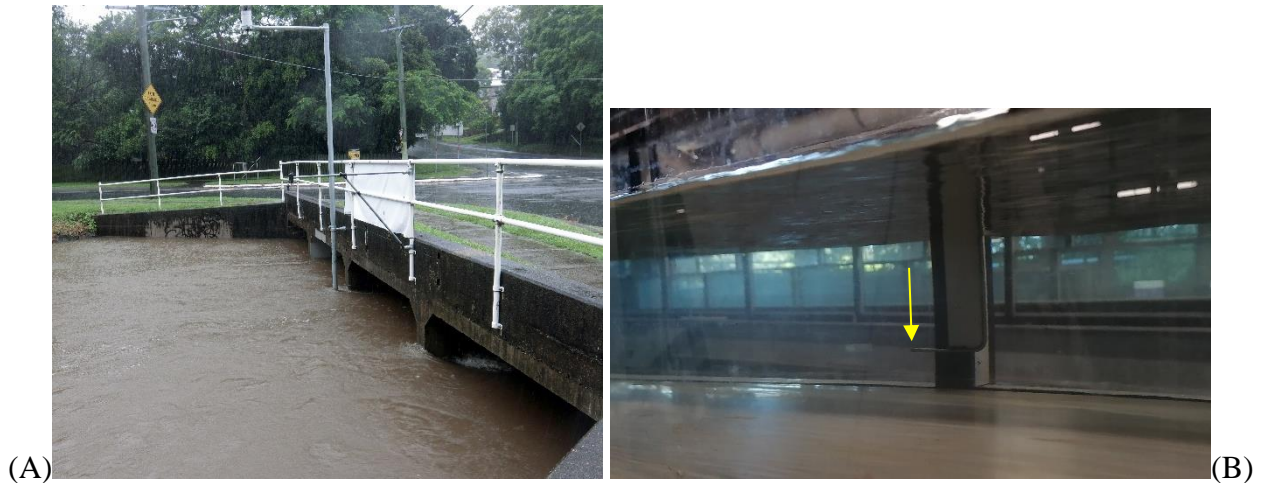
Figure 1 , Culvert channel. (A) Prototype culvert in Indooroopilly, Australia during a large flood in February 2024. (B) Experimental facility at the University of Queensland with Prandtl-Pitot tube in operation (yellow arrow) – Flow direction from left to right in both photographs.
