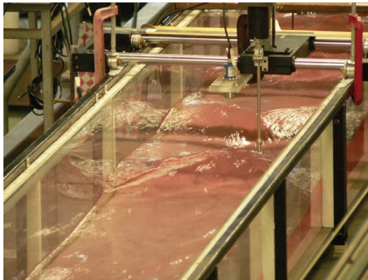
(A) Undular tidal bore ( Fr = 1.4 , Q = 0.040 \text{ m}^3\text{s}^{-1} , d_0 = 0.08 \text{ m} )
