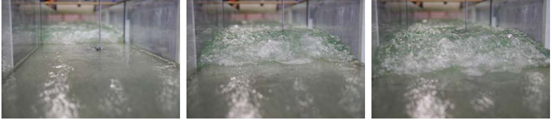
Figure 2 Breaking bore propagation in laboratory, looking downstream ( Fr_1 = 2.1 )
